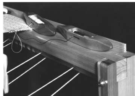
i. The cloth protector is raised 1" above the breast beam to act as a barrier for falling shuttles. Add a piece of 1/4" dowel before inserting the cloth protector in the slot.
