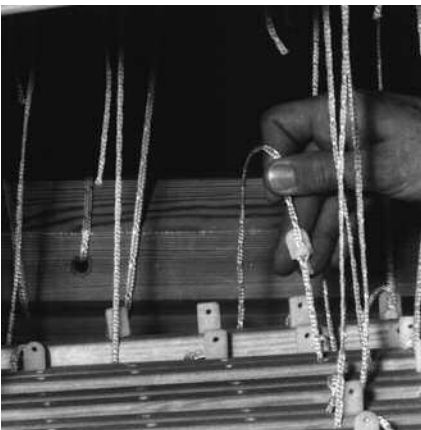
f. When changing to a new tie-up, re-do only the cords for shafts that do something different. Insert the Texsolv clip the appropriate number of notches away from taut for each shaft: four notches for shaft 4 in a 10-shaft tie-up.
